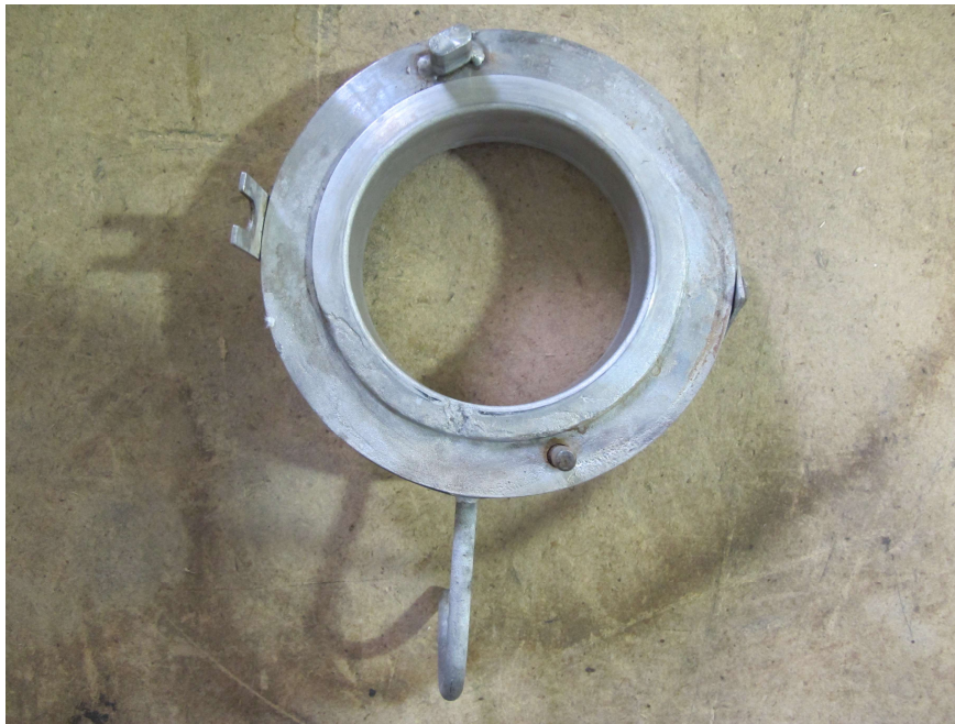
Figure 49—Rupture Disk Holder Subjected to Corrosion
