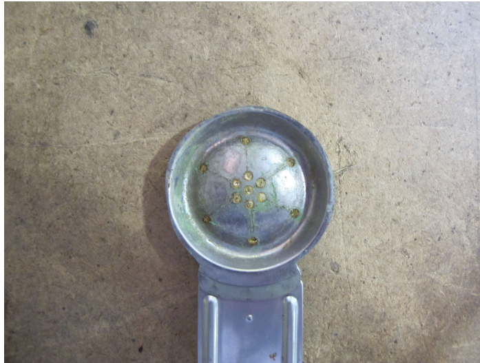
Figure 46—Disk Subjected to Corrosion
