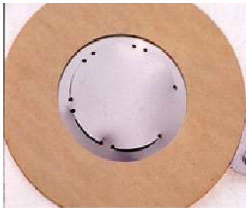
Figure 45—Operating Ratio Exceeded—Tabs Are Stretched
