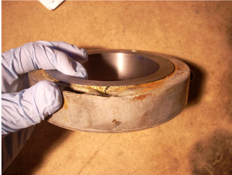
Figure 50—Rupture Disk Holder Corrosion Due to Leakage
