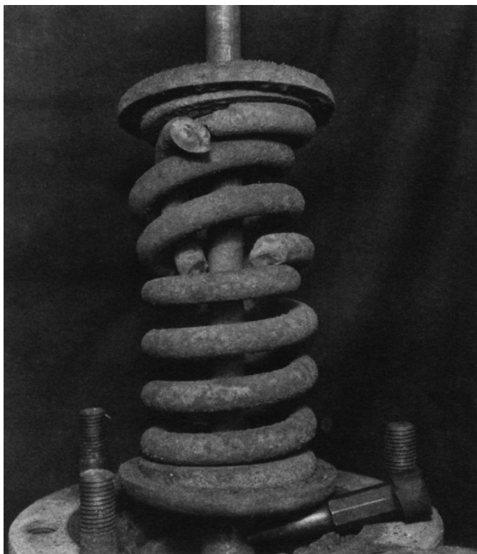
Figure 30—Spring Failure Due to Corrosion
