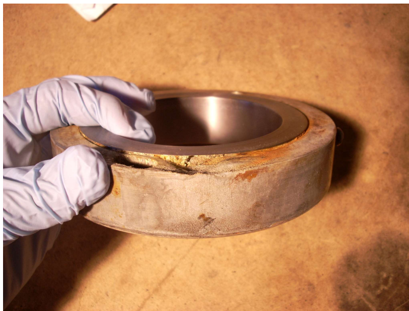
Figure 50—Rupture Disk Holder Corrosion Due to Leakage
