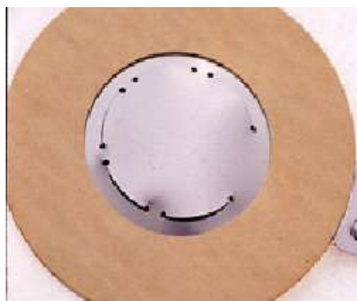
Figure 45—Operating Ratio Exceeded—Tabs Are Stretched
