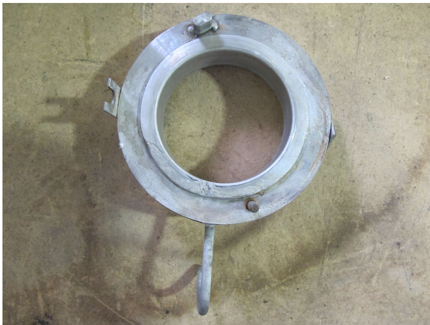
Figure 49—Rupture Disk Holder Subjected to Corrosion
