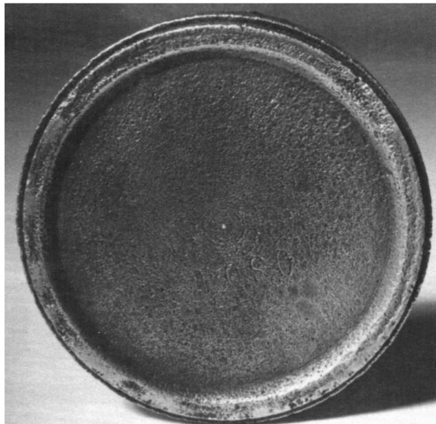
Figure 24—Chloride Attack on 18Cr-8Ni Steel Disc
