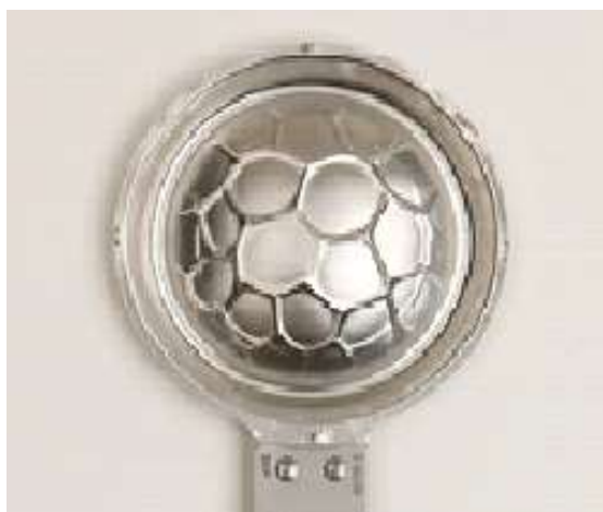
Figure 44—Operating Ratio Exceeded, Then Subjected to Vacuum
