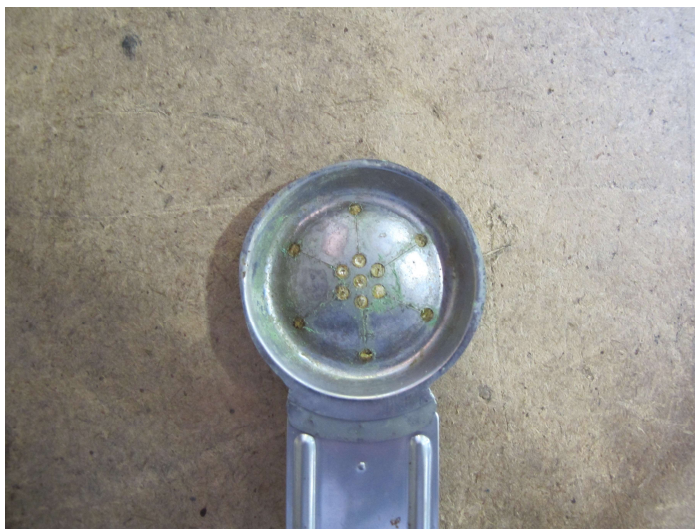
Figure 46—Disk Subjected to Corrosion
