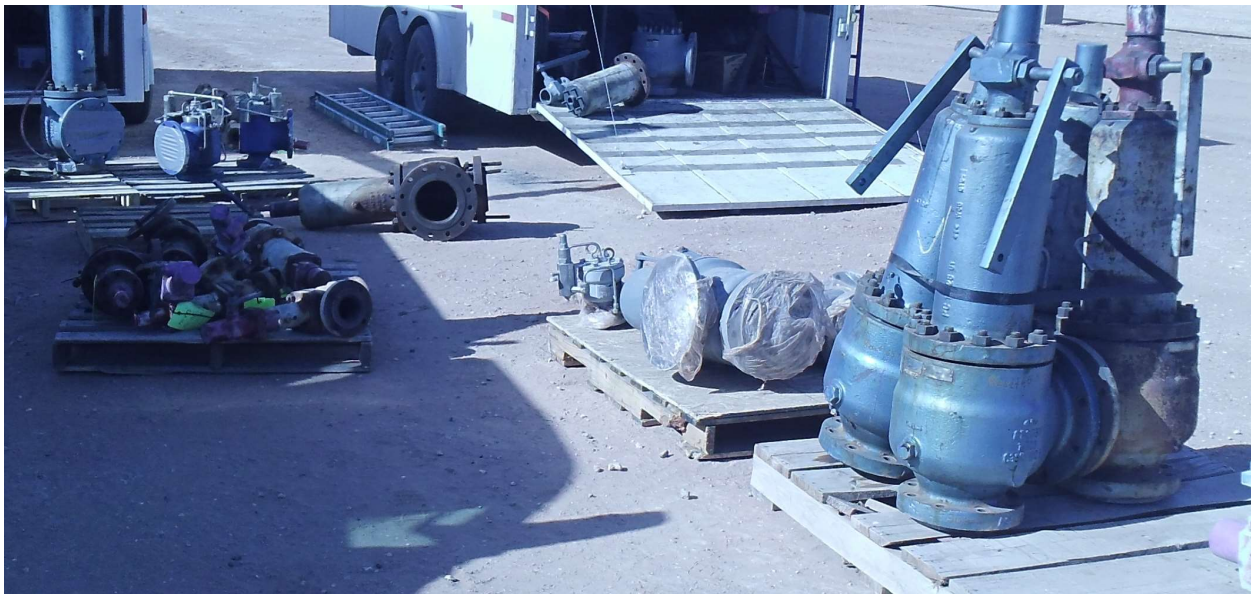
Figure 37—Example of Improper Storage of Valves
