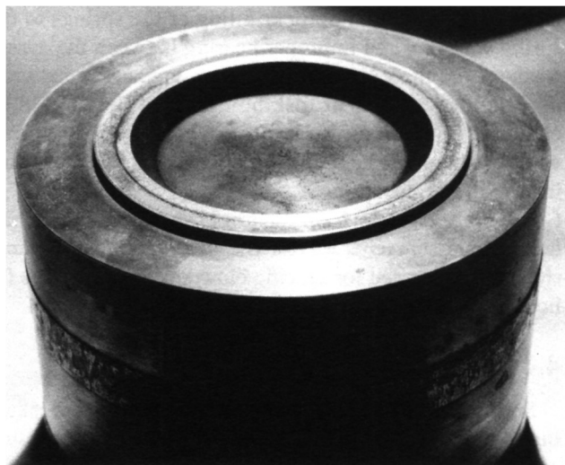
Figure 28—Seating Surface of Disc Deformed by Chattering
