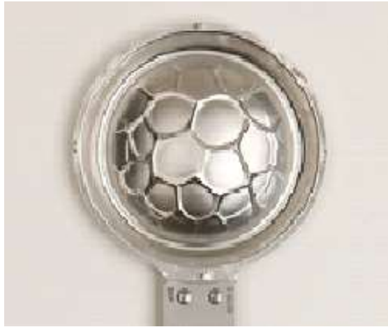
Figure 44—Operating Ratio Exceeded, Then Subjected to Vacuum
